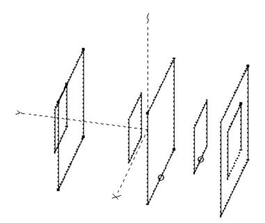
The sketch shows the element arrangement with the reflectors aligned. The 80-meter array is about 111' long, while the 40-meter array is about 118' long. The designs use AWG #12 copper wire.
