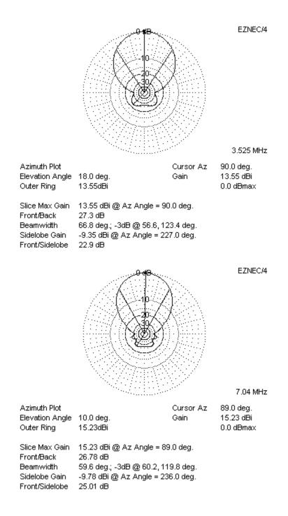
The patterns show that there is very little interaction between the two arrays, which are assumed to have separate feedlines.
