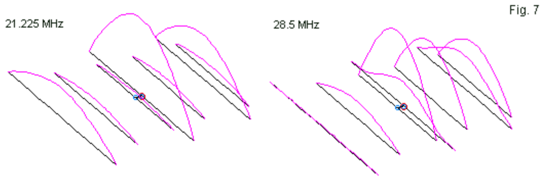
Relative Current Magnitudes on the Elements of a Dual-Band Yagi at Different Frequencies
