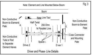
Since you need only 24.6" of phase-line (plus a bit of extra for connections to the elements), you likely should make your own. The following table lists the center-to-center spacing for  $250-\Omega$  lines using some common bare copper wires, listed by AWG size.
