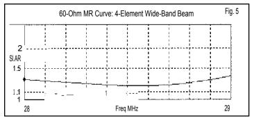
The phasing system that uses 2 driver elements does not produce a deep SWR null, that is, 1:1. However, it is designed to show a very low figure at every operating frequency within the first MHz of 10 meters.
